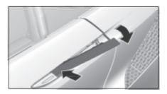
By switching the auto pop-out main switch to OFF, you can disable the auto pop-out function. For the purpose of safety and to prevent damaging the vehicle, disable this function and manually operate the handle, especially when the vehicle is being shipped by train, truck, or boat.
