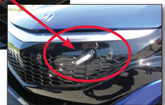
Tow eyelet inserted into front bumper location
