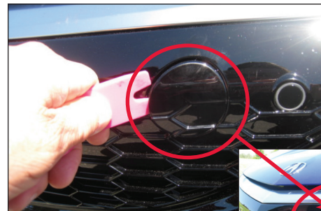
Remove cover from front bumper with plastic trim device
