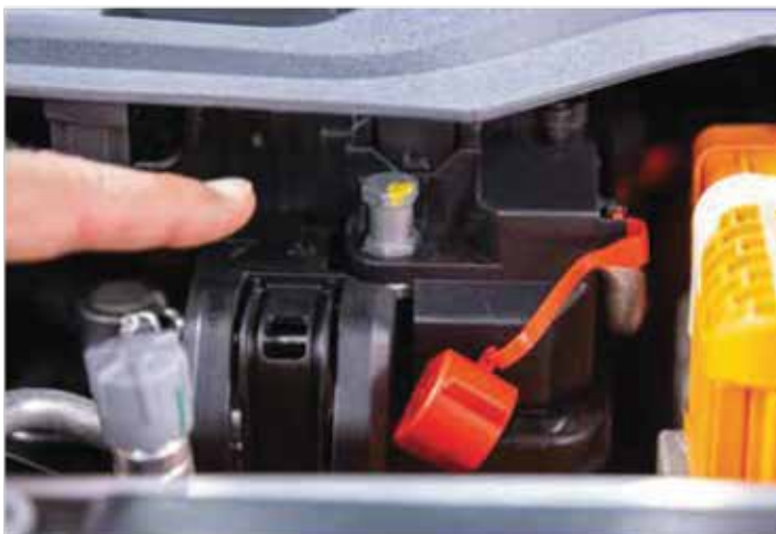
Remove red cover at positive jump post to make connection.
