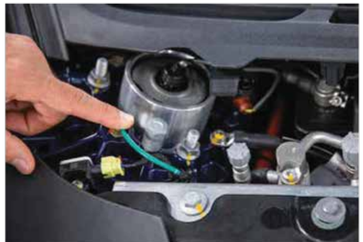
Make connection at negative jump post.
