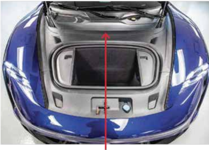
In front trunk area, remove cowl compartment cover.
