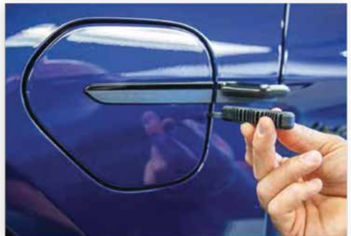
Insert the removal tool in the center of the rear side of the charge door.
