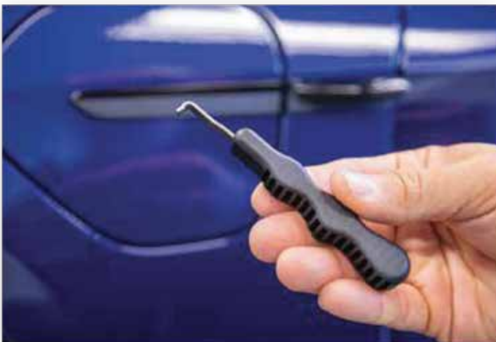
Charge door removal tool.
