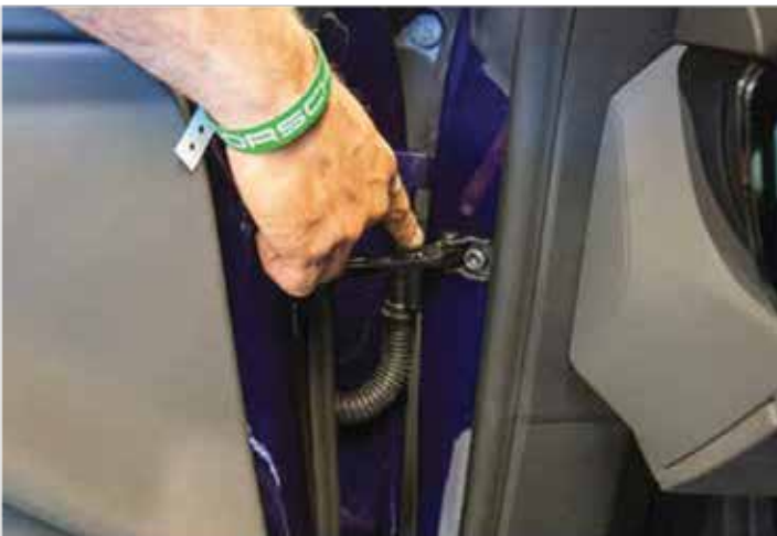
Make the 12-volt negative connection at the door check on the driver side door.
