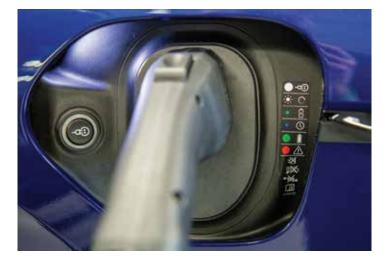
In the unlikely event that the charging plug refuses to disengage from the charging port, there is a mechanical release available to free the plug on either side of the vehicle.
