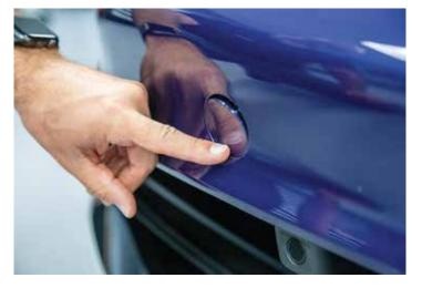
Front eyelet cover – press in at the bottom.
