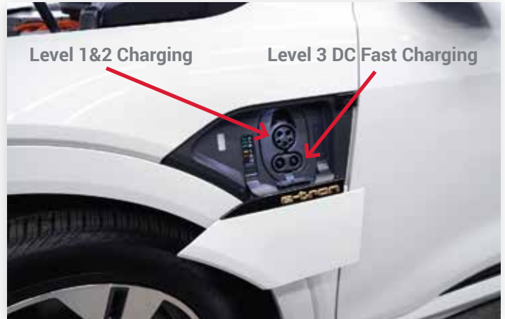
Driver Side Charge Door Level 1/2 & Level 3 DC Fast Charge Capable
