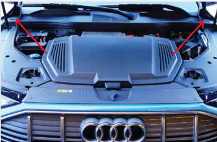
Manual Charge Door and Charging Cord Releases can be found in the cowl area for each charge port assembly
