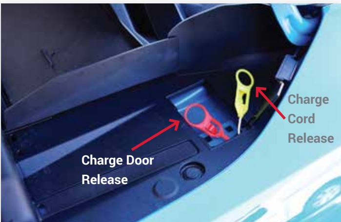
Manual Charge Door and Charging Cord Releases can be found in the cowl area for each charge port assembly
