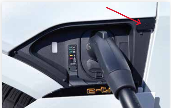
Driver Side Charge Door Level 1/2 & Level 3 DC Fast Charge Capable
