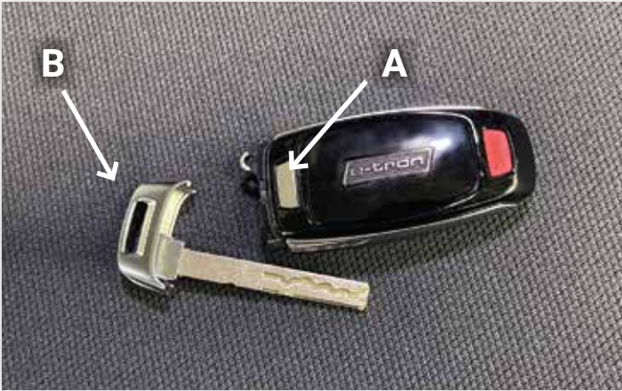
Press button on back side of Key Fob (A) to remove mechanical key blade (B)
