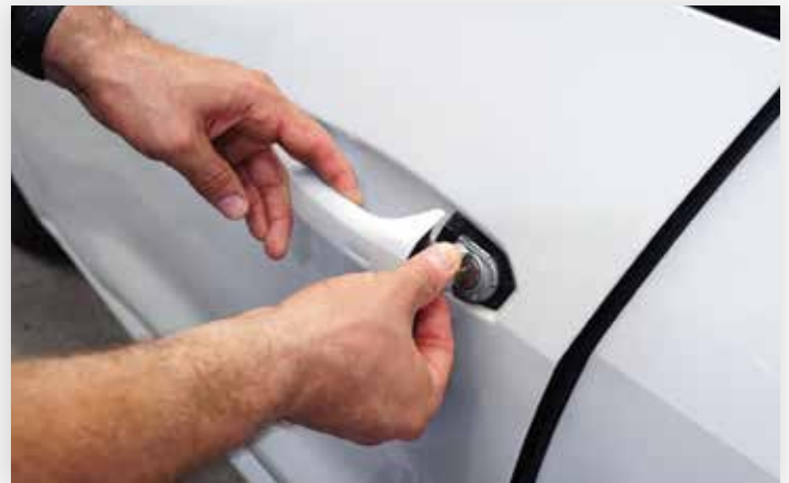
With Key Blade turned fully Counter Clockwise firmly pull handle to open door.
