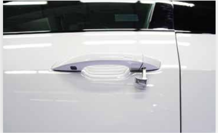
Insert Key Blade in slot in lock cylinder cover. Gently pull forward on key blade to remove cover.
