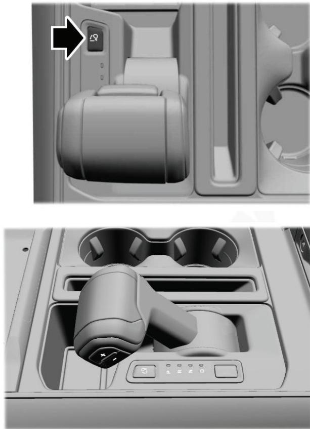
**Note:** Do not store objects in the selector lever stow bin, and be sure that the bottom selector lever tray mat is flat inside the selector lever stow bin.
