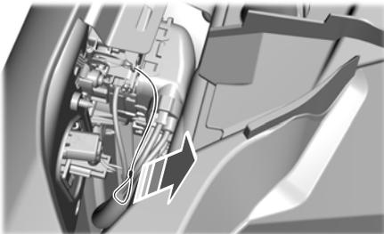
7. Remove the charge coupler from the charge port.
