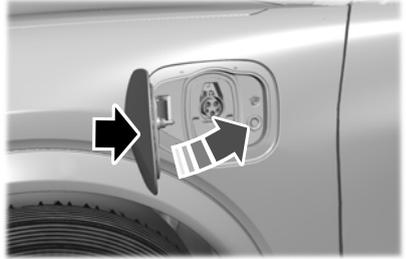
3. Press the center right-hand edge of the charge port door to close.
