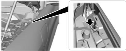
6. Between the gap of the hood and windshield, access the manual release mechanism and pull the pull ring firmly, perpendicularly towards the center of your vehicle. Once pulled, make sure you do not tangle the pull ring cord as it resets on the next charge session.
