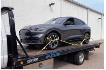
Retain and transport only using 8-point carrier kit
