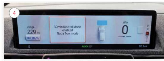
Prior to activating "Neutral Mode" make all connections to tow truck to prevent roll away.
