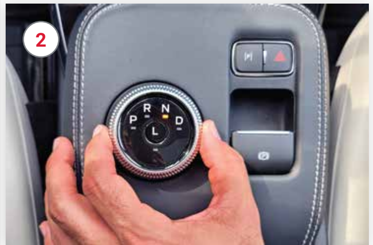
Shift the vehicle from P (Park) to N (Neutral) while holding both pedals all the way down.
