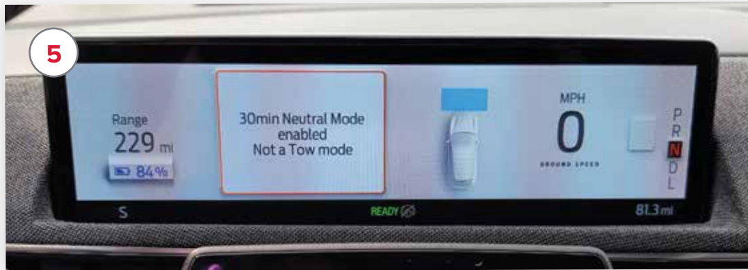
Vehicle will enter ‘Neutral Mode’ for 30 minutes as indicated in dash information display
