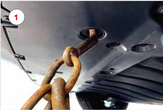
1 Make connections to the disabled Mustang Mach-E at the round openings under front bumper
