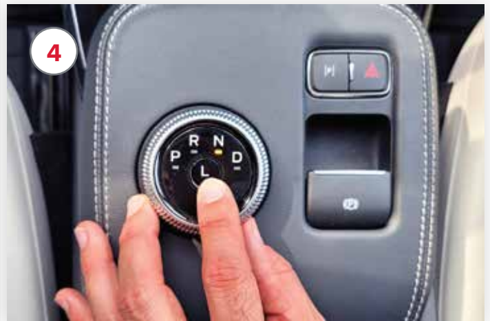
4 Press 'L' in center of rotary shifter
