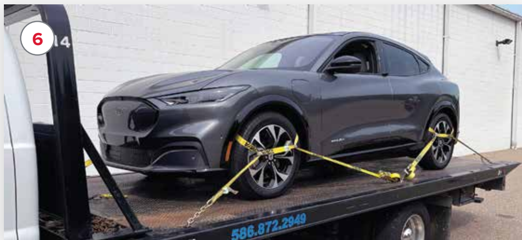
Load vehicle to Rollback Tow Truck for transport, 8 Point Retention ONLY
