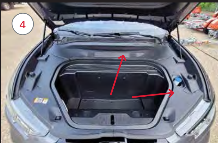
Cowl & driver side trim panels will need to be removed. No tools are required.
