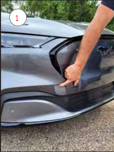
Remove panel in front bumper pressing at top to remove from bumper cover.
