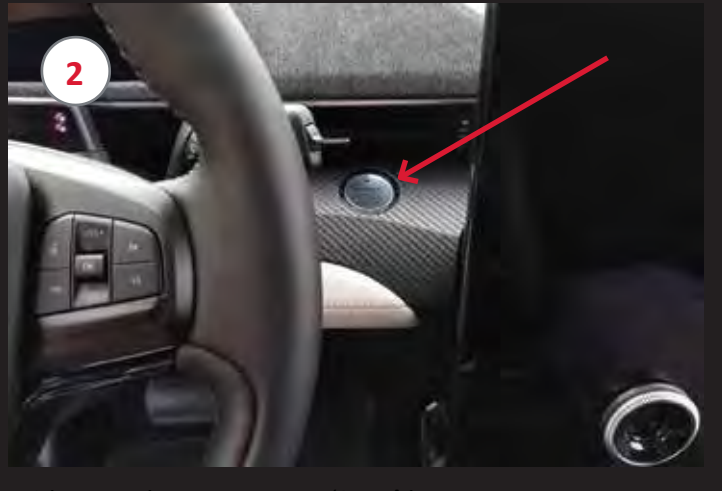
2 With Key Fob present press 'Start' button to power up vehicle
