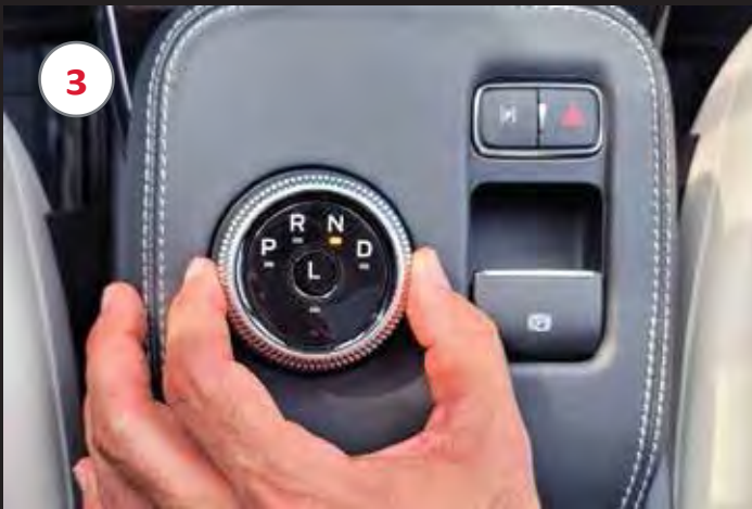
3 Shift vehicle to 'N' Neutral with rotary shifter in center console
