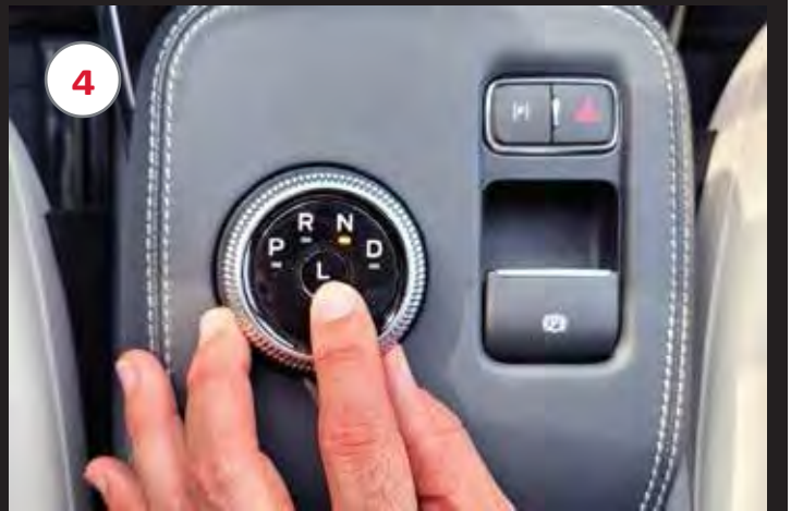
4 Press 'L' in center of rotary shifter
