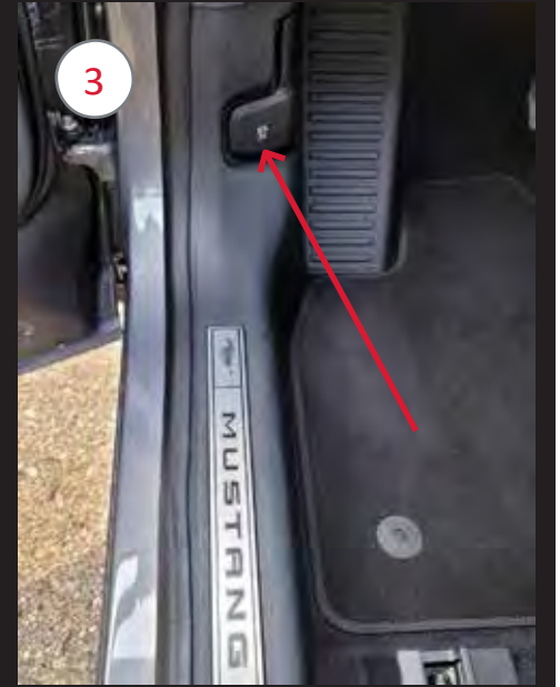
Pull front luggage compartment release twice to fully release front cover for opening.
