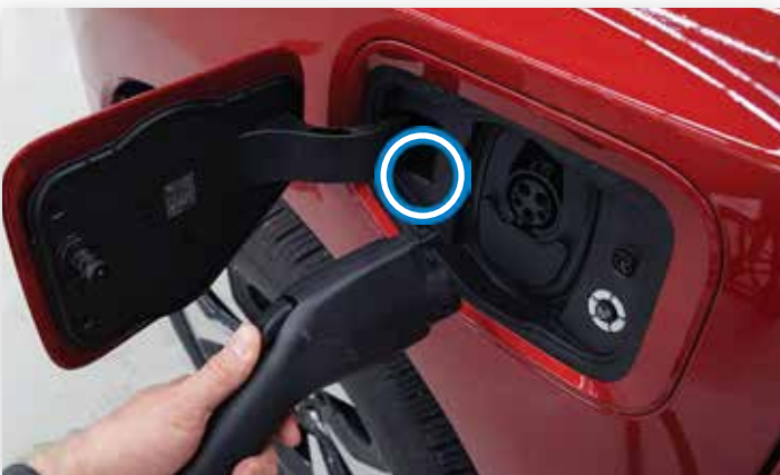
While pulling up on the release cable press latch on back of the charge coupler to disengage from charge port.
