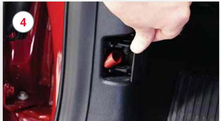
Emergency Manual Release - Driver's Kick Panel
