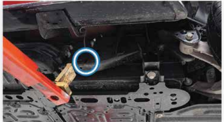
Driver side rear frame rail jacking location
