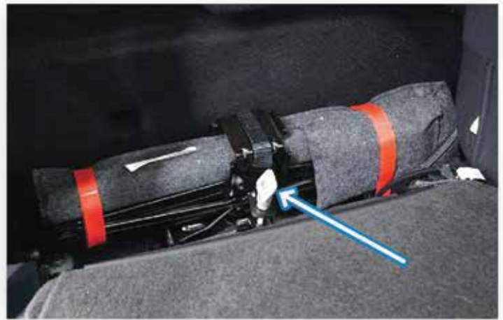
Remove wing bolt to access jack and tool kit
