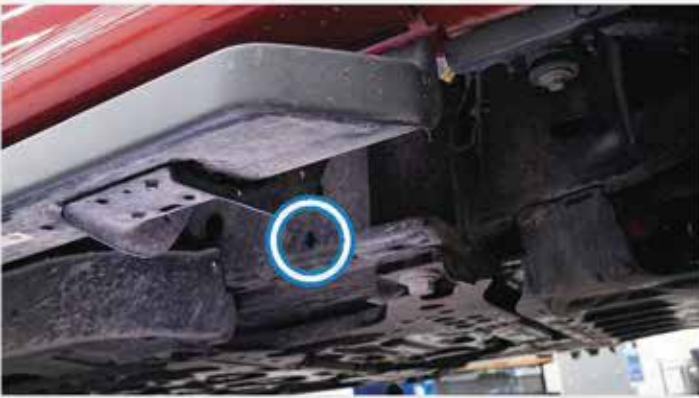
Passenger side front frame rail jacking location
