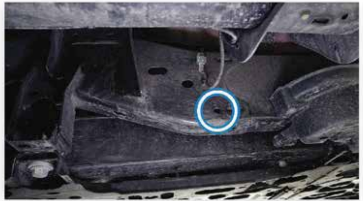
Passenger side rear frame rail jacking location
