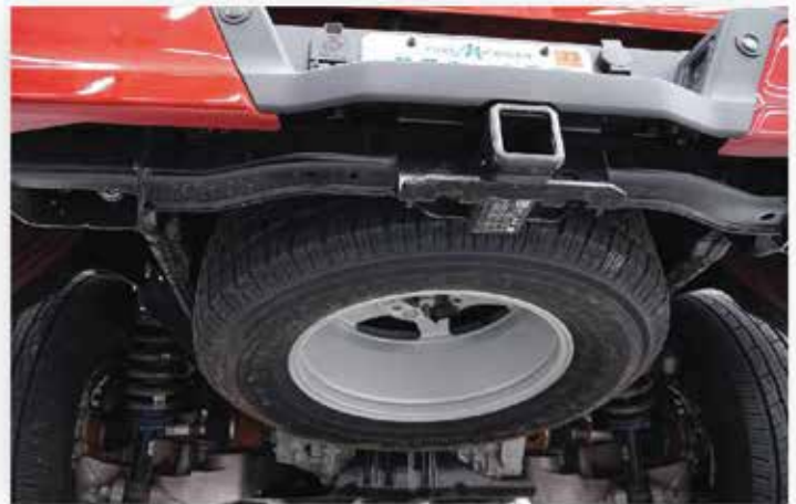
Assemble jack handle slip joint rods to lower spare tire at rear
