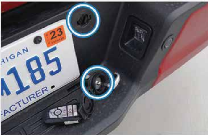
Mechanical key from key fob is needed to remove lock cylinder
