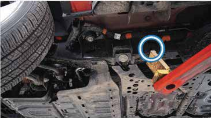
Driver side front frame rail jacking location
