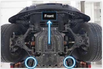
Make connections to the disabled F-150 Lightning at the transport slots in the bottom of the frame behind the sway bar mounts
