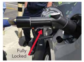
Lift lever fully to locked position. Nozzle must be fully locked to fitting to prevent disengagement during filling.
