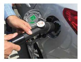
Firmly press nozzle onto fitting to engage connection.
