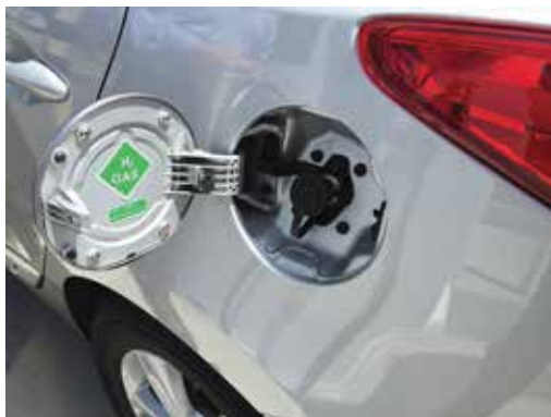
Green hydrogen gas decal and fitting in filler door
