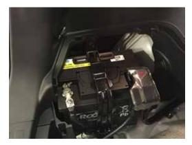
Connect jump box to the battery Power up vehicle with the "POWER" button on the dash to the right of the instrument cluster.
