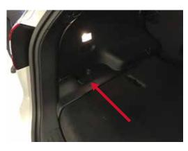
The vehicle's 12-volt battery is located in the cargo area at the left rear corner.
