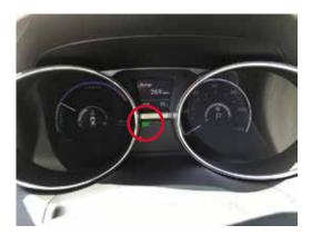
When the green "READY" light illuminates in the dash cluster, the jump box can be removed and the vehicle is ready for operation.
