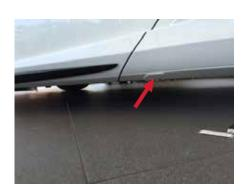
The cover in the driver's side rocker panel will need to be removed. Pull the latching tab forward on the rear edge of the panel. Rotate down and pull toward the center of the vehicle to free the cover.
