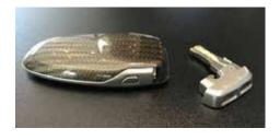
This mechanical key can only open the driver's side door.
