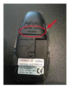
The battery cover can be removed with a coin or finger nail on this lip.
