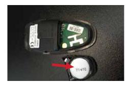
Pay close mind to battery orientation for reinstallation of new unit.
