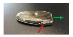
To manually open the door on the 650S the mechanical key will need to be retrieved from the fob.
