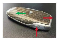
First press button on side of fob and remove mechanical key from the fob
