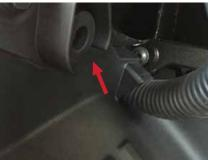
The "Bonnet" or Front Cargo Cover can now be opened with the manual release found in the driver's lower door opening to gain access to the compartment housing the Lithium Ion start battery.
