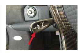
Prior to navigating the left hand display any error massages or reminders will first need to be acknowledged. These faults are stored and can be recalled at any time; acknowledgement does not mean they have been erased. On the left hand side of the steering column, below the turn signal stalk, is the control stalk for the left hand display.
