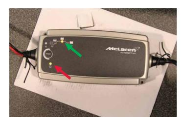
With the 12 volt supply cord plugged into the receptacle on the car next plug the charger into the wall socket.
