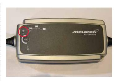
If the charge level in the lithium ion start battery of your McLaren v650S falls below given threshold, it will go into "sleep mode" and need "waking up". The illumination of the error light on the charger indicates that the battery has reached this level of discharge.
