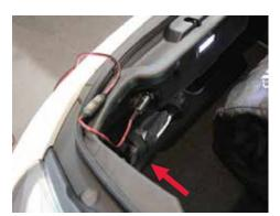
Locate the corresponding plug for the 12 volt supply going to the vehicle and plug into the charging port located on the driver's side of the cargo area Charging the 650S with the supplied charger is the easiest and least invasive manner in which to bring the Lithium lon start battery back to a full charge.
