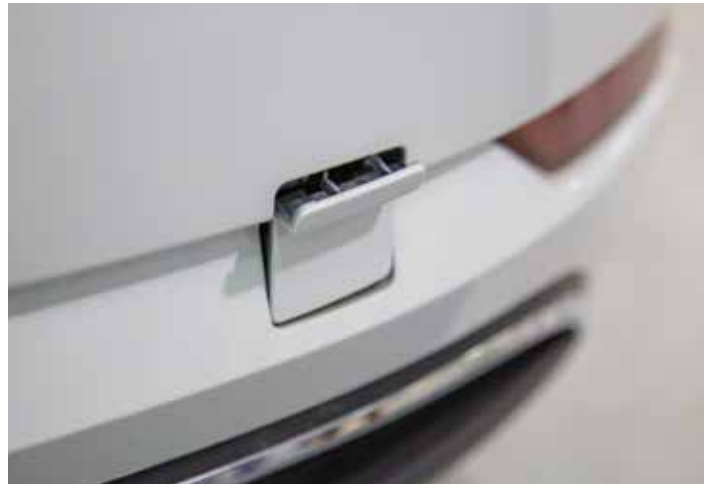
REAR: Press the bottom of the rear eyelet cover to remove.
