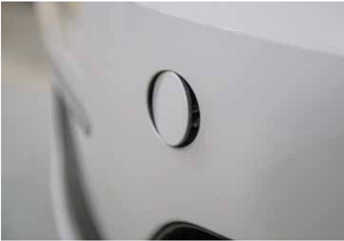
FRONT: Press the left side of the front eyelet cover to remove.
