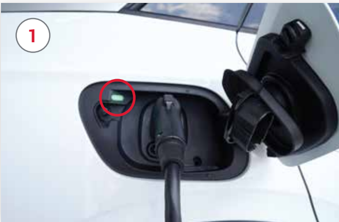
While charging, the charge status light will pulse green and plug cannot be released.
