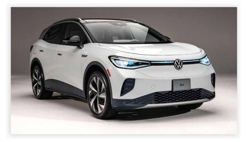
Weight – 4559 lbs - 4683 lbs Drive Architecture – Rear Drive or All Wheel Drive No Tire Inflator Kit Free Roll Mode available when vehicle is charged - No Mechanical Park Override Front Tow Eyelet – Left-hand thread Rear Tow Eyelet – Not Available on some vehicles Mechanical Key Cylinder in drivers door 8-Point Carrier Retention ONLY Level 1/2/3 charging
