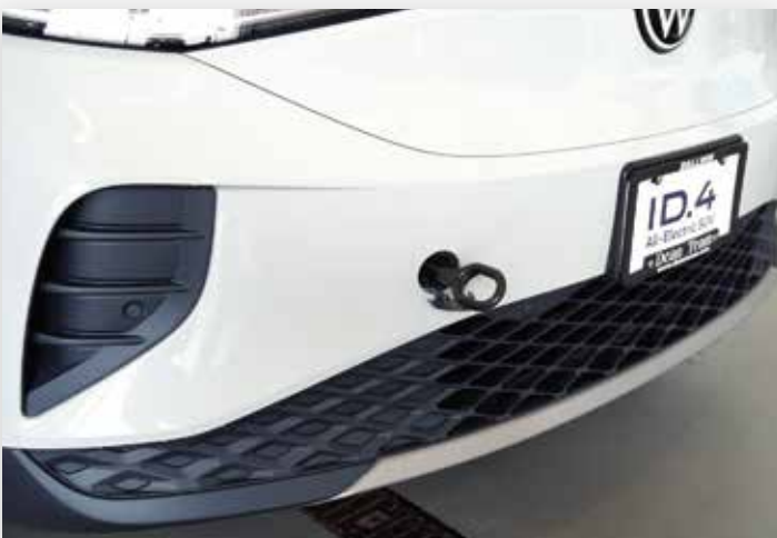
Tow eyelet is left-hand thread
