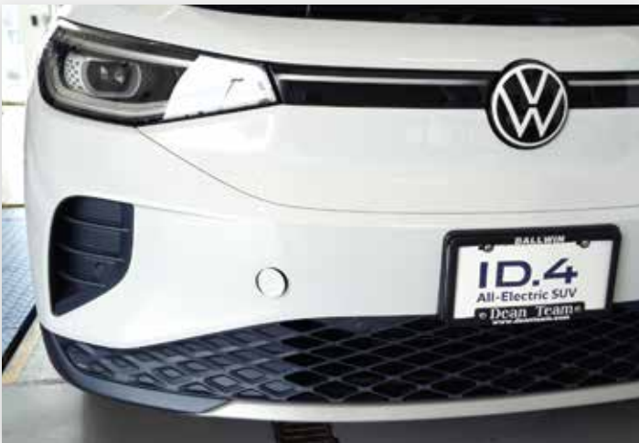
Tow eyelet provision in front bumper
