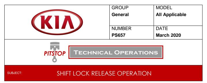
This Pitstop provides information regarding a no-start condition due to a dead battery. It is recommended to jump start, or charge the battery in order to move the vehicle. If this is not possible, follow the procedure below to utilize the 'Shift Lock Release' button to move the shift lever from Park (P) to the Neutral (N) position. Refrain from forcing the vehicle out of Park (P) by pulling aggressively on the shift lever.
