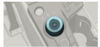
Put the vehicle in P (Park) position by pressing the 'P' button on the rotary shifter
