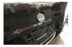
Press in on top of tow eyelet cover to remove.
