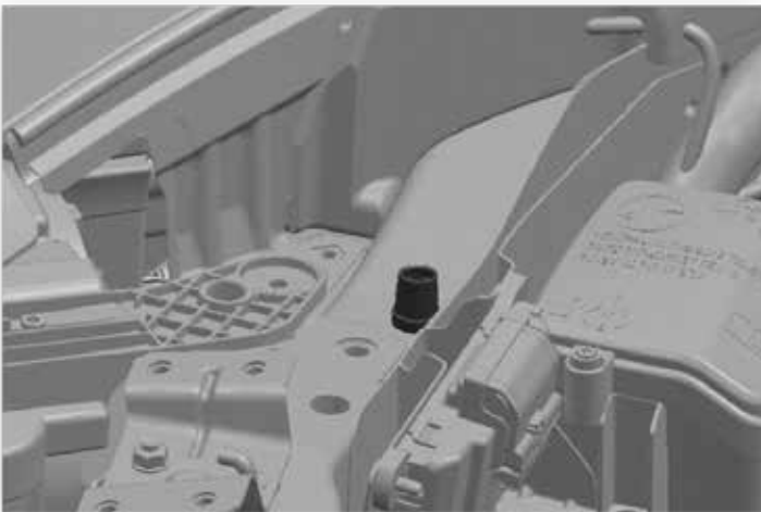
Remote Negative (-) Post Location
