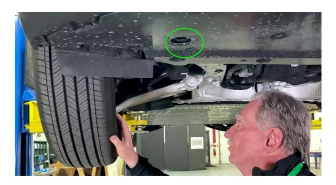
The Mach-E can be pulled using the Front Winching Holes. This would mean that the operator would run the winch line under the rear of the vehicle all the way up to the front winching holes.
