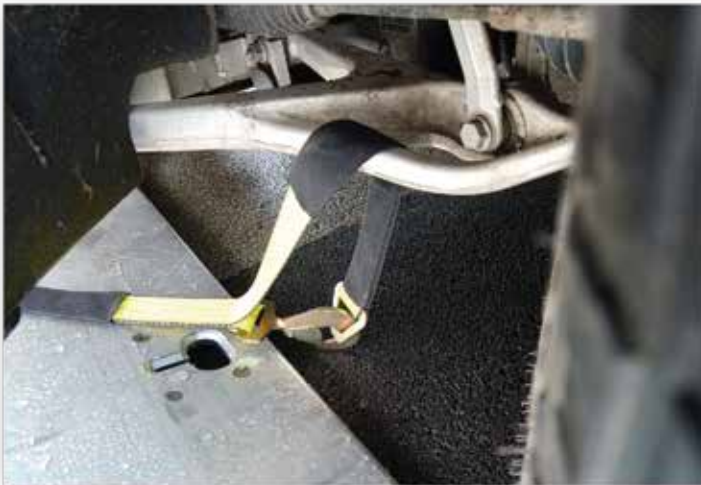
Connection Points for Loading to Rollback Tow Truck are at the Front Control Arms with a Nylon Wrap Around Style Bridle (Shown)
