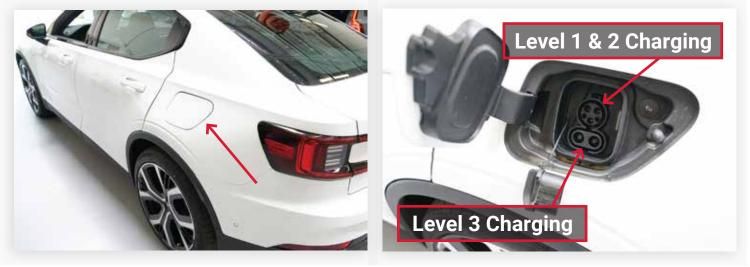
The Charge Door on Polestar 2 is on the driver side quarter panel. Press in on the rear part of the door to open.
