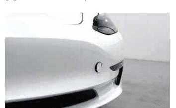
Remove Tow Eyelet Cover to access remote jump leads
