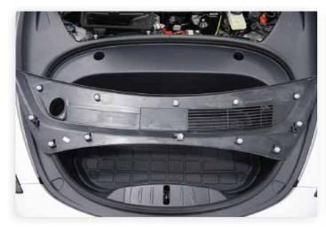
Verify all fasteners are intact and reinstall Service Panel in cowl.
