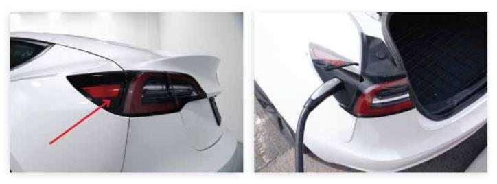
With the vehicle unlocked the charge port door can be opened by pressing it at the bottom
