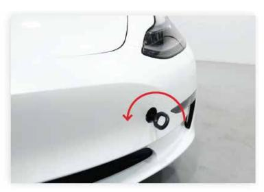
Tow Eyelet is left hand threaded, install counterclockwise until its fully seated in the bumper beam.
