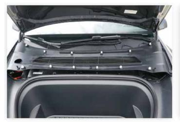
Verify all fasteners are intact and reinstall Service Panel in cowl.
