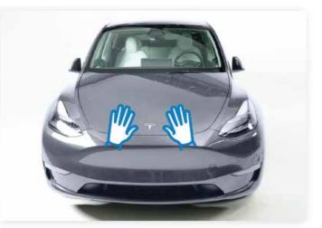
Pressing it closed elsewhere may damage the panel.
