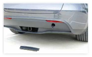
Tow Eyelet is left hand threaded, install counterclockwise until its fully seated in the bumper beam.
