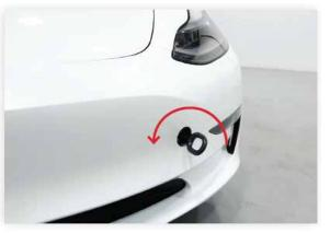
Tow Eyelet is left hand threaded, install counterclockwise until its fully seated in the bumper beam.
