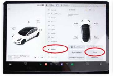
In order to place the Model Y into Transport Mode 12 volt power and detection of a key are required. Vehicle must be powered up
