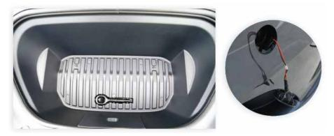
\* Vehicles with no Low Voltage Power, the front trunk can be accessed via the two small jump leads on the back of the Tow Eyelet Cover
