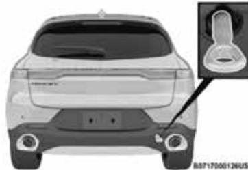
Rear Tow Eye Installed
