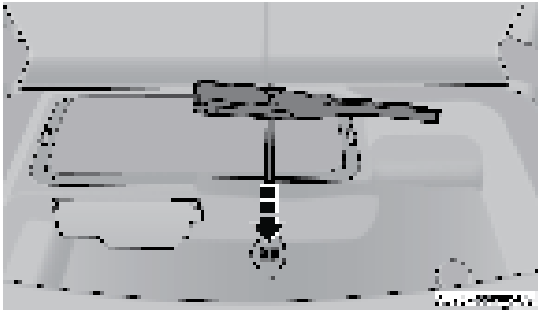
Winch Drive Nut Location
