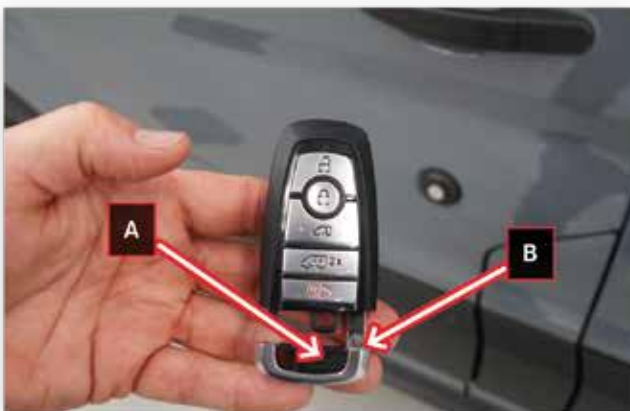
Press button on front of Key Blade (A) to remove mechanical key blade (B)
