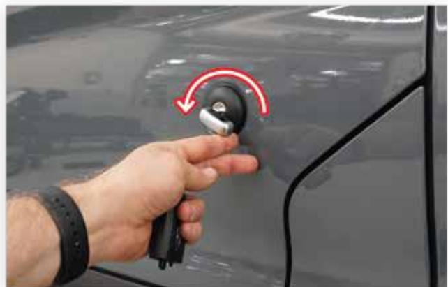
Insert Key Blade in Lock Cylinder Rotate Counter Clockwise, pull handle to open
