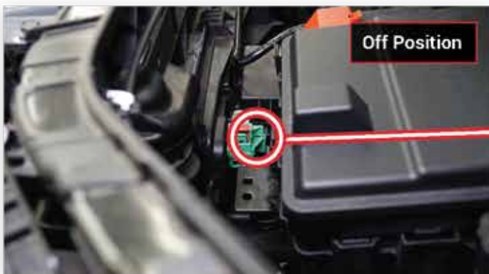
Locate Charge Coupler Release and Low Voltage Service Disconnect
