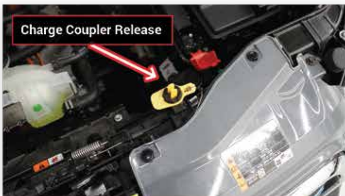
Locate Charge Coupler Release and Low Voltage Service Disconnect
