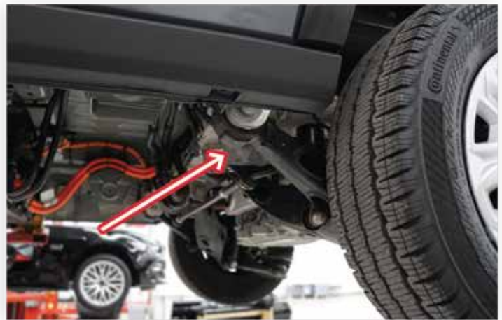
Rear jacking location, in front of rear tire, outer bush of suspension arm reinforced pad
