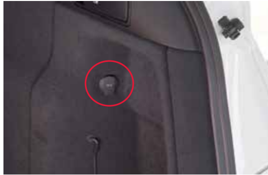
12-volt power source in the cargo area
