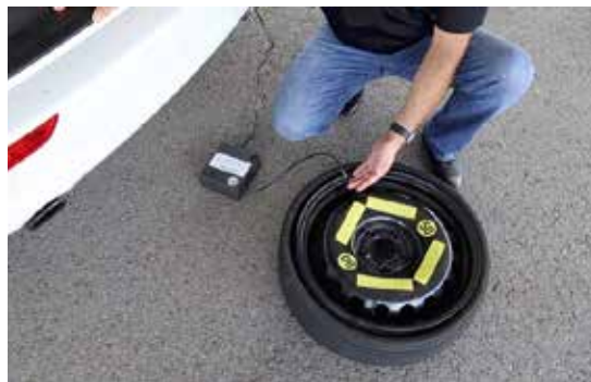
Connect the air line to the valve stem, then plug in the compressor to the power source.
