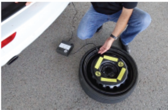
Connect the air line to the valve stem, then plug in the compressor to the power source.
