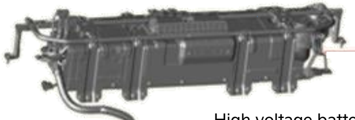
High voltage battery
